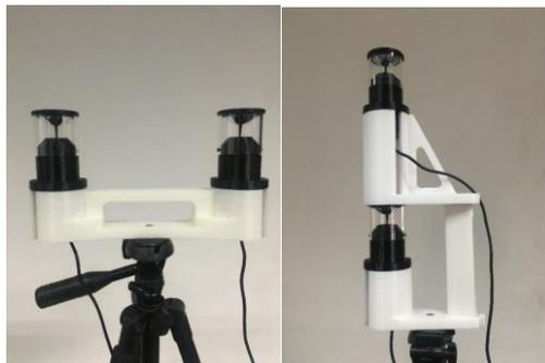
**Figure. 5.** Horizontal camera design (a) and vertical design(b).
