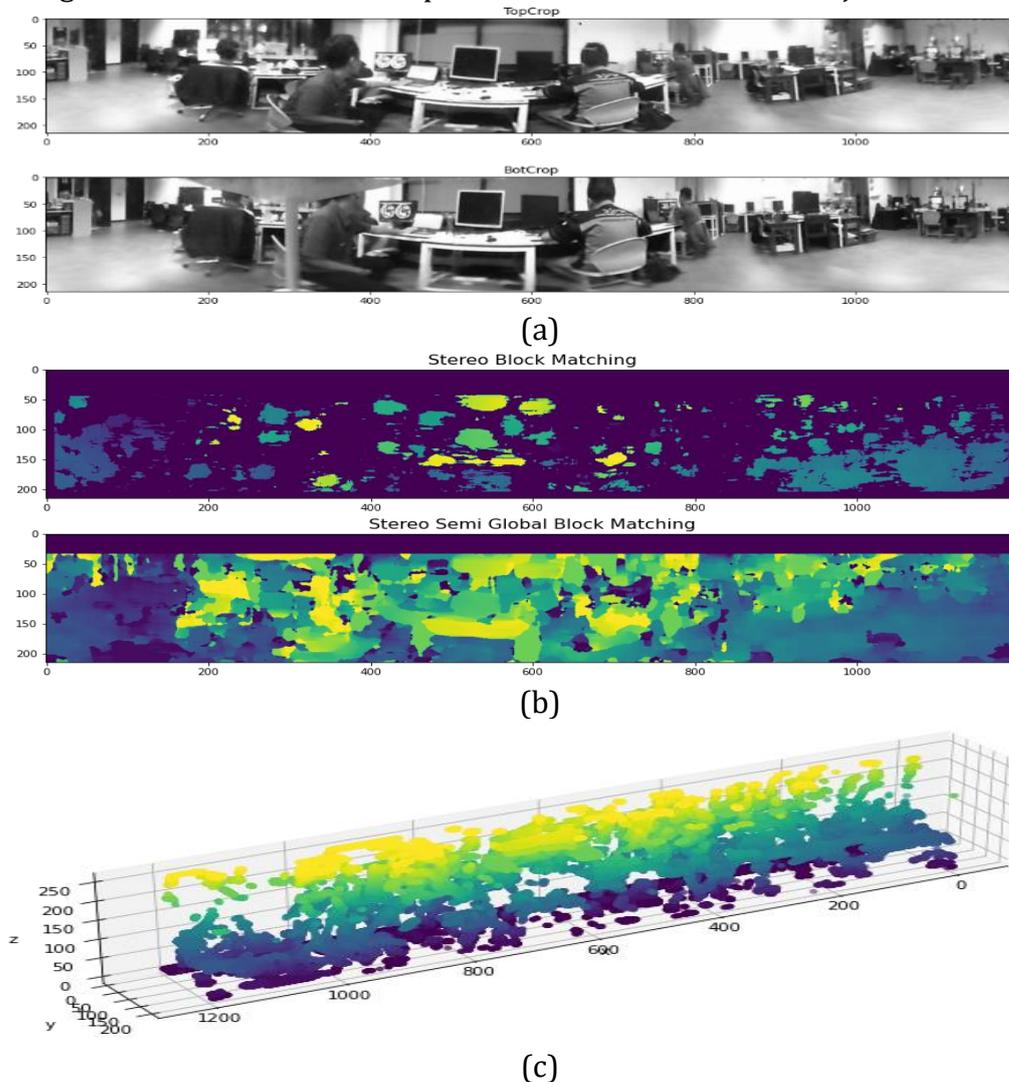
**Figure. 9.** The results of vertical stereo matching from top and bottom camera (a), using the BM and SGBM (b), and shown with 3D visualization (c).
