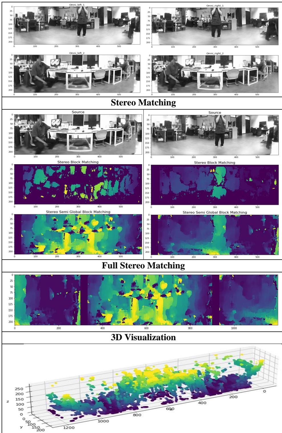
Figure. 10. Horizontal Stereo Matching.
