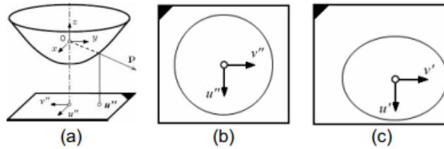
**Figure. 1.** Omnidirectional coordinate system (a), Sensor plane with matrix coordinate(b), Camera image plane with pixel coordinate that depends on affine transformation.
