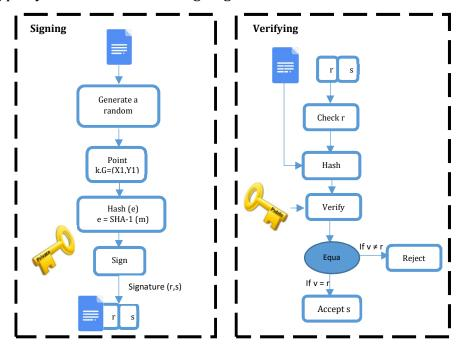
Figure 1. ECDSA cryptosystem in signing mode
