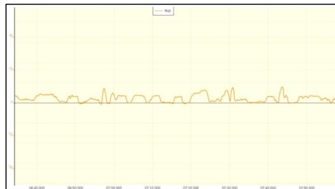
Figure 11b. Experimental roll angle response under conditions of low wind disturbance and payload
